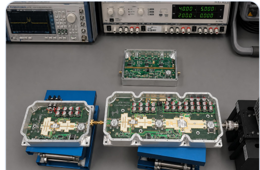
Figure 3.6 — Cascaded HPA Modules During Laboratory Evaluation.
