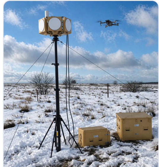
Figure 3.1 — Field-deployed counter-UAV RF detection setup with antenna hardware, support equipment, and an airborne UAV target.
