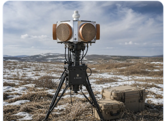
Figure 3.2 — Field-deployed directional antenna concept for RF sensing and bearing-support functions in a counter-UAV environment.
